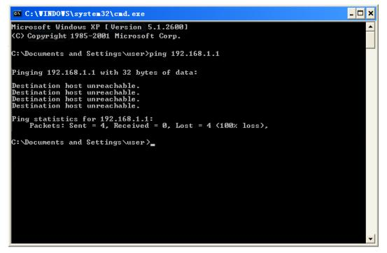
Figure 3-2 Failure result of Ping command
