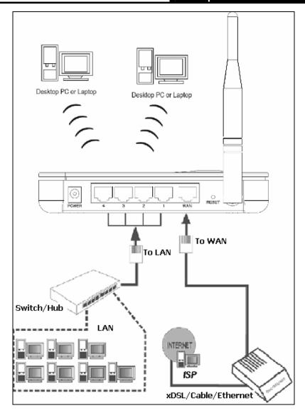
Figure 2-3 Hardware Installation of the Router
