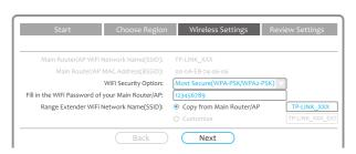
c. Fill in the **Wi-Fi Password of your main router/AP**. TL-WA854RE's **Wi-Fi network name (SSID)** can be copied from your main router/Al **(TP-LINK\_XXX)** or be customized **(TP-LINK\_XXX\_EXT)**.
